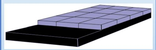
Distresses like rutting and cracking, which are predominant in case of asphalt pavements can be avoided with help of whitetopping. Some other advantages include lower maintenance, lower life cycle cost compared to asphalt overlays. Also as concrete is relatively light in colour, it absorbs less heat and reduces the urban heat island effect.
