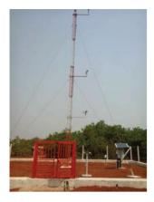
The School of Earth, Ocean and Climate Sciences of the Institute in association with Indian Space Research Organization (ISRO) has installed and operationalized the Mini Boundary Layer Mast (MBLM) at the Argul Campus. It is one of the observation premises out of 28 such installations being step up all over the country
