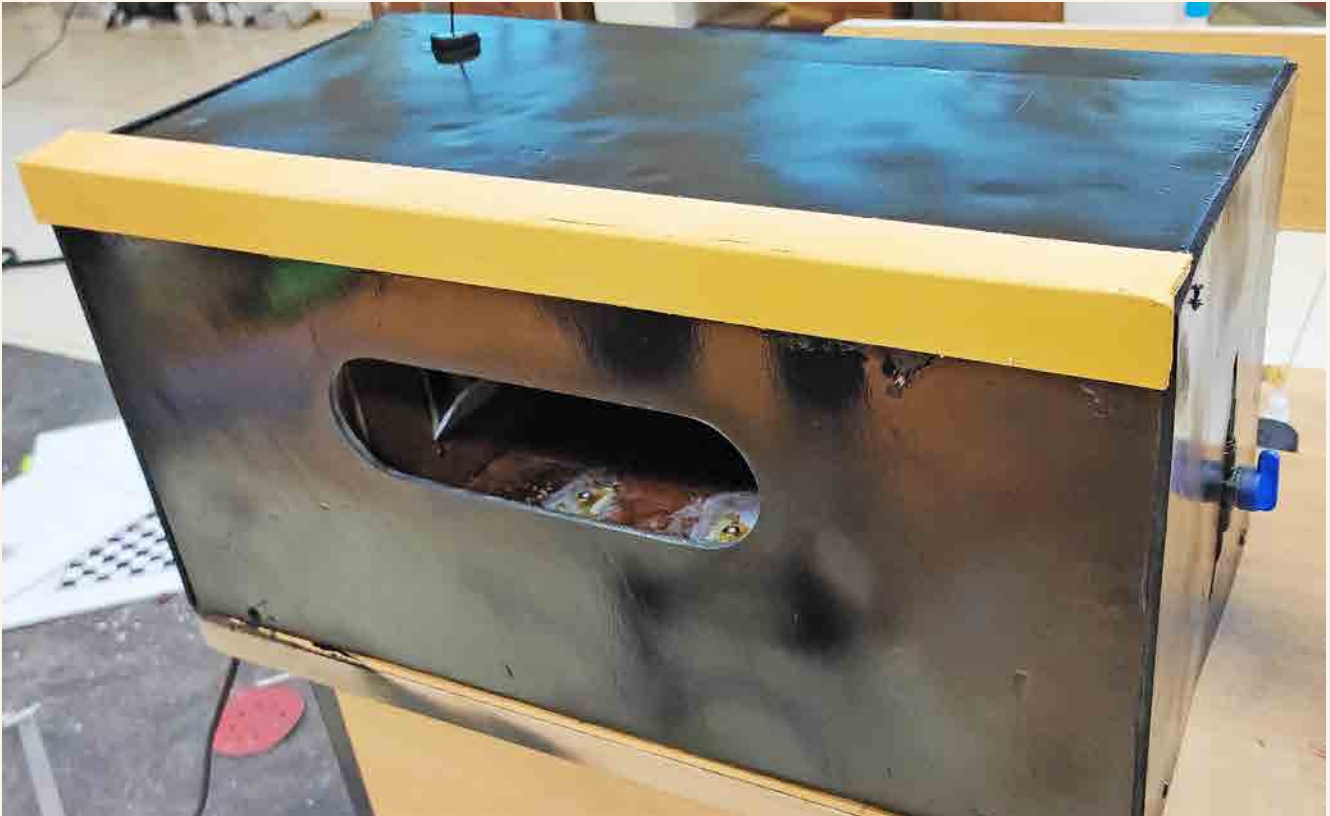
Version 1: Automatic Hand Sanitizer with its own pump system, container & misting technology for industrial use.
