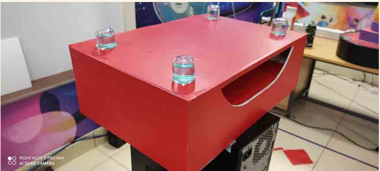
Version 2: Automatic Hand Sanitizer with its own pump system, container, misting technology & rechargeable battery pack for personal use as well as industrial use
